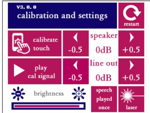
Press the “restart” button at the top right of the screen to restart the device once you are done making adjustments.
