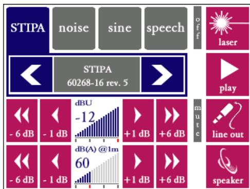
Select any of the tabs on the top-left bar to access any of the four categories of test signals: Speech intelligibility (STIPA), Noise, Sine or Speech. Then choose the test signal which you need for your measurements. Consult chapter 4 of this manual for further explanations on the different types of test signals.
