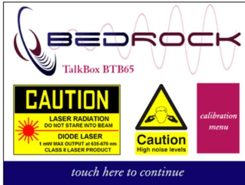
Press on the blue bar at the bottom of the screen to skip directly into the main menu. Press the button “calibration menu” if you need to adjust the level calibration of the TalkBox or to change any of the hardware settings. See section 3.3 for a description of these settings.
