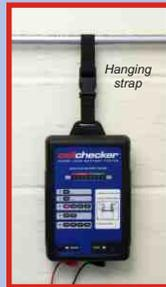
The hanging strap has a quick release buckle for easy fastening to conduit, pipes, ladder rung, etc.
