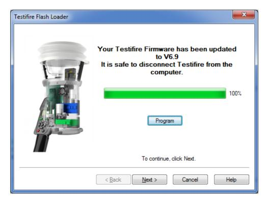
In the unlikely event that the programming process fails or programming is aborted by the user, Testifire remains in Boot Loader mode. Click "Cancel" to continue to exit the program. Then disconnect the USB cable and Battery Baton from Testifire. The programming process can then be repeated from Step 1.
