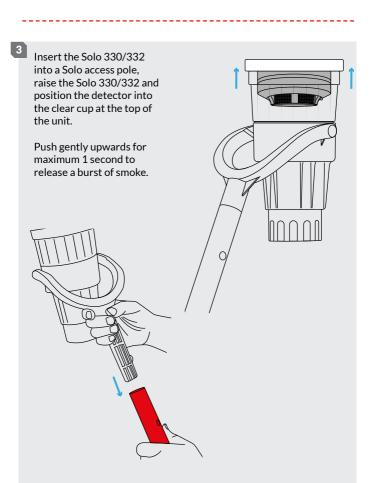
Repeat every 10 seconds without removing the detector for maximum of 1 minute until the detector is activated. On alarm, remove cup to allow particles to disperse.
