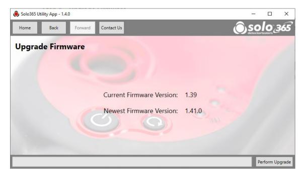
Once the upgrade begins, the main LEDs on your Solo 365 will turn orange and will return to flashing green once the upgrade is completed.
