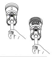
Lower Testifire once the heat test has completed. Testifire will return to idle.
