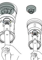
heat and CO are tested at the same time in a simultaneous test. Once the alarm is triggered lower Testifire. Testifire will return to idle with the same settings - ready for the next simultaneous test.
