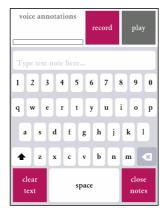
Text notes are saved in a text file (.TXT), voice notes in a .WAV file - each with the same serial number as the current measurement. Voice annotations can be recorded either through the measurement microphone or a headset microphone (connected through the headset jack on the side of the device). The input channel can be selected in the "Settings" module.
