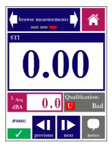
"Settings" screen and "browse measurements" screen. The latter screen is nearly identical to the STI measurement screen, but with previous/back buttons instead of start/stop and save buttons.
