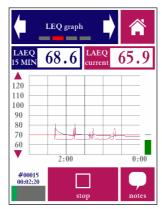
Screen 2 of the LEO module, showing a graph of how the average LAEO is developing.
