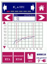
R'w (left) and STC (right) measurement result based on the measured D and the shifted reference curve (show in graph). Note that first RTA spectra need to be selected in screen 2 before these data can be calculated.
