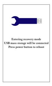
The device can now be accessed through USB. This means you can copy a new .EAP update package to the UPDATES folder. If you are having trouble accessing USB in the normal operating modes of the AM100, this may be a way to restore your system and reinstall the latest firmware.
