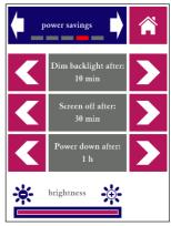
Left: measurement settings (measure continuously and start delay Right: power saving settings (backlight time-out and display brightness)
