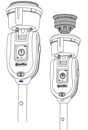
The test will begin automatically when the tester cup is placed over the detector, breaking the infrared beam. The status LFD will flash to indicate the choosen test application has started.
