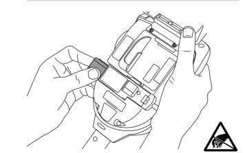
Slide the smoke cartridge completely into the smoke
