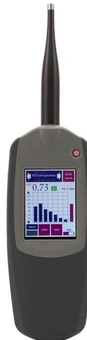
Bedrock SM50 is a versatile speech intelligibility tester for fire safety systems. It has a user-friendly touch screen for easy control and can measure both STIPA and full STI. Features include RTA, FFT, Reverberation Time, Noise Curves, and more. It also has a USB port for quick connectivity and includes a hard case.
